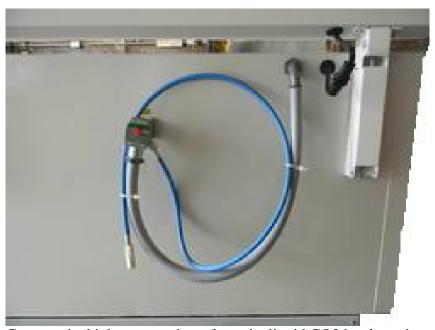
Connect the high pressure hose from the liquid CO2 bottle to the solenoid valve on the rear of the freezer using an 1/8" MPT to 1/4" flare stainless steel fitting.
